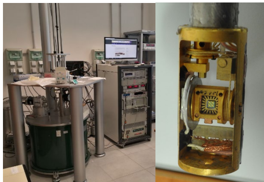
Cryogenic superconducting magnet (10.5 T, 0.3-300 K)
