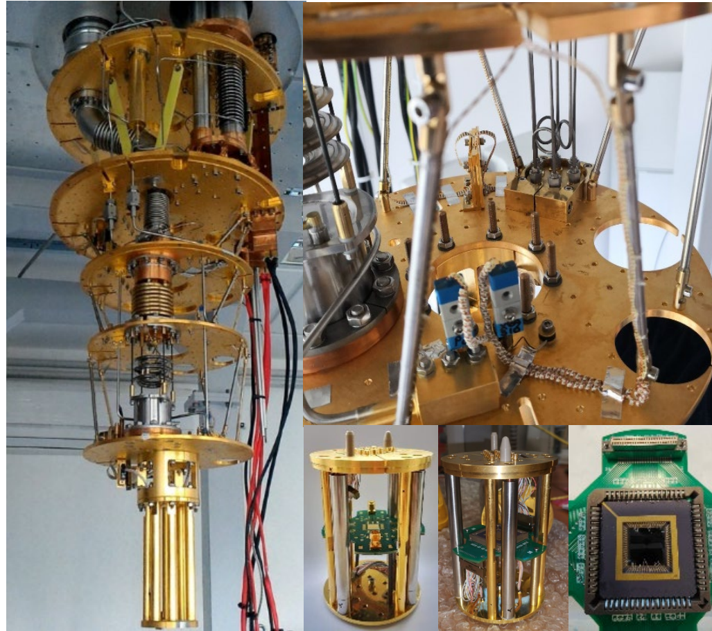
Oxford dilution refrigerator (down to 10 mK, vector magnet 6T/1T/1T)
