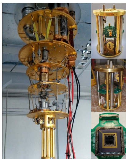
Oxford dilution refrigerator (down to 10 mK, vector magnet 6T/1T/1T)
