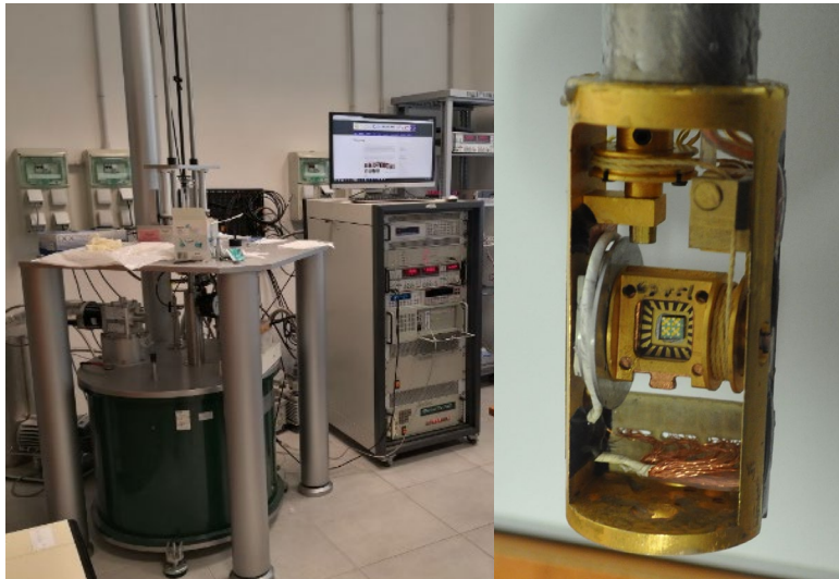
Cryogenic superconducting magnet (10.5 T, 0.3-300 K)
