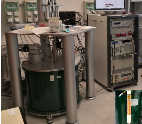
Cryogenic superconducting magnet (10.5 T, 0.3-300 K)
