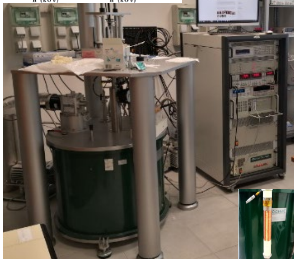
Cryogenic superconducting magnet (10.5 T, 0.3-300 K)
